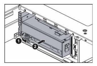
7 Lift the locking tab (3) on the back of the tape drive tray, then push the tape drive (4) and tape drive bracket out of the tray.
